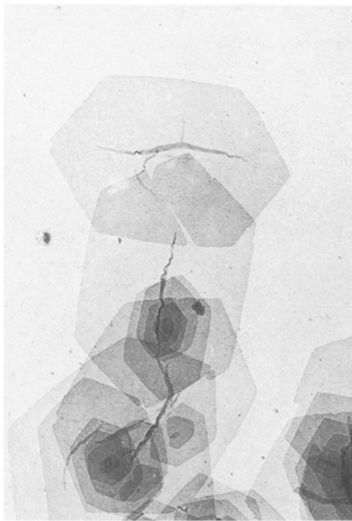
Figure 1 Single crystal of polyethylene grown from 0.05% solution in octane at 93° C. The central pleats indicate that the crystal has collapsed from its original three-dimensional structure ( \times 7800 ).
